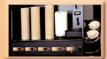
Internal view of 3 selection plus sugar dispenser machine
